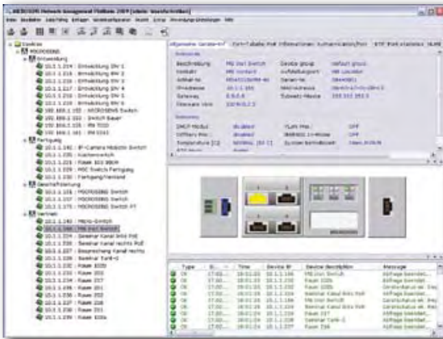
Network tree structure, device status and Event-Manager
