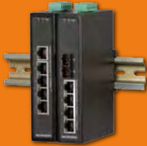
Fast Ethernet Switches with 4x PoE
