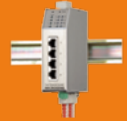
Fast Ethernet Industrial Switch with ring function
