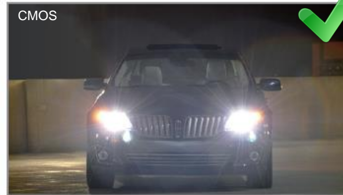
No smearing with CMOS sensor
