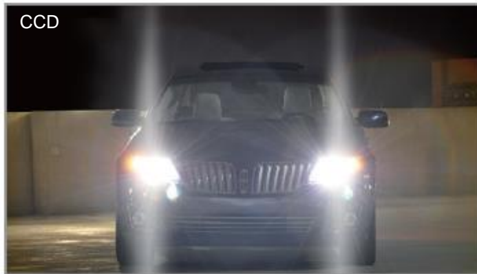
Vertical smearing originated from headlights at night
